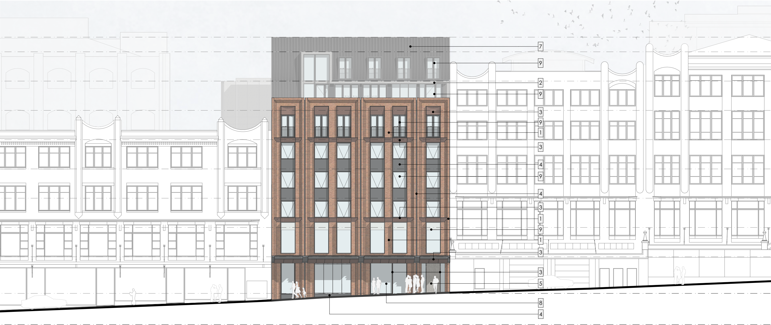
1. BRICK WALLS & BREEZEWAYS RECLAIMED BRICK IN RED TONES TO MATCH LOOK OF READERS DIGEST BRICKS
